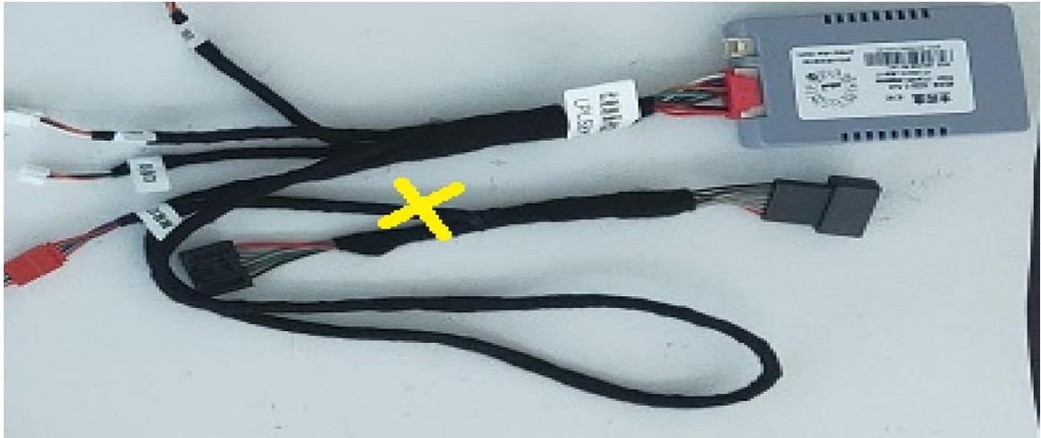
Find the 32P cable of the left main engine on the front passenger side of the original vehicle. My green "CAN-L" cable is Connected to The "second" pin cable of the original "32P". ( You need to remove a bit of the "second" pin plastic casing. Then my green "CAN-L" cable is soldered to the "second" pin. )
