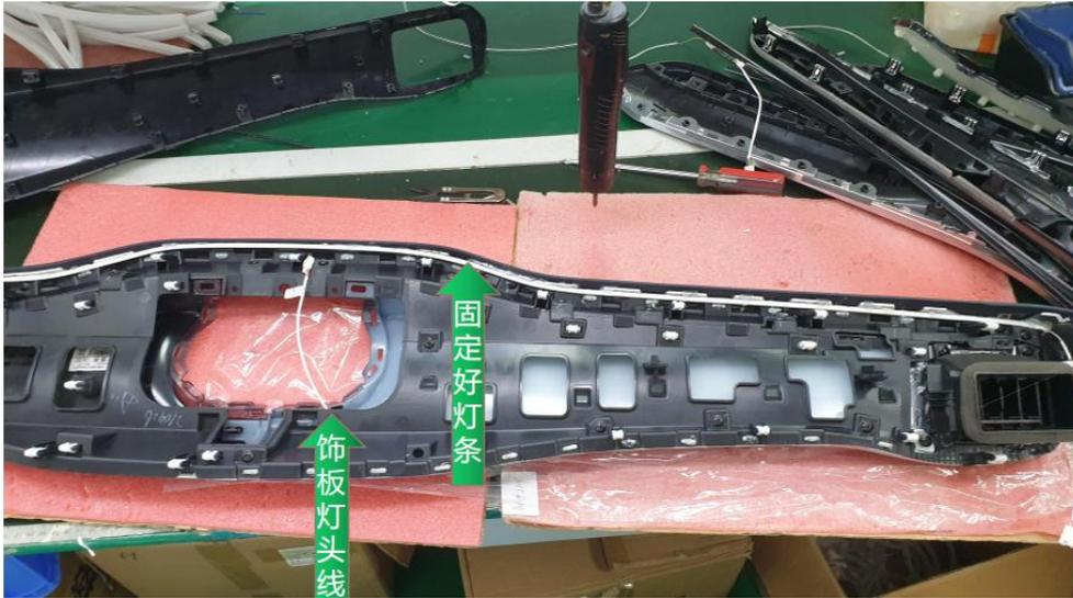
7. Install the light under the saddle.
