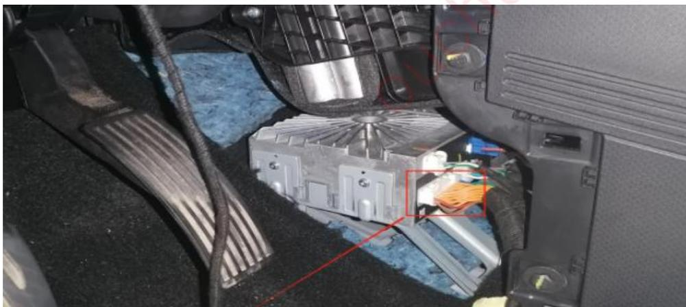
My **Brown "CAN-H"** cable is Connected to The **"31st"** pin cable of the original **"32P"**。 (You need to remove a bit of the **"31st"** pin plastic casing. Then my **brown "CAN-H"** cable was soldered to **"31st"** pin ) 。
