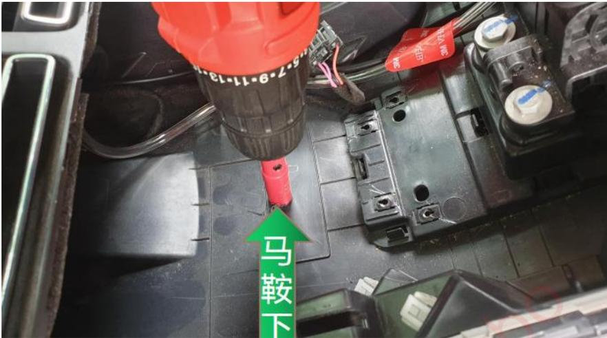
8. Install the front light of the gear lever.
