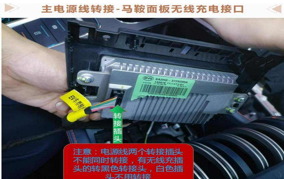
4. If the original car does not have a "wireless charging connector", you need to Cut off my power cable at the "yellow" marked position. Then manually connect the "CAN" cable. Then you will see 4 cables. (Red "ACC" cable. Green "CAN-L" cable. Brown "CAN+H" cable. Black "GND" cable.)
